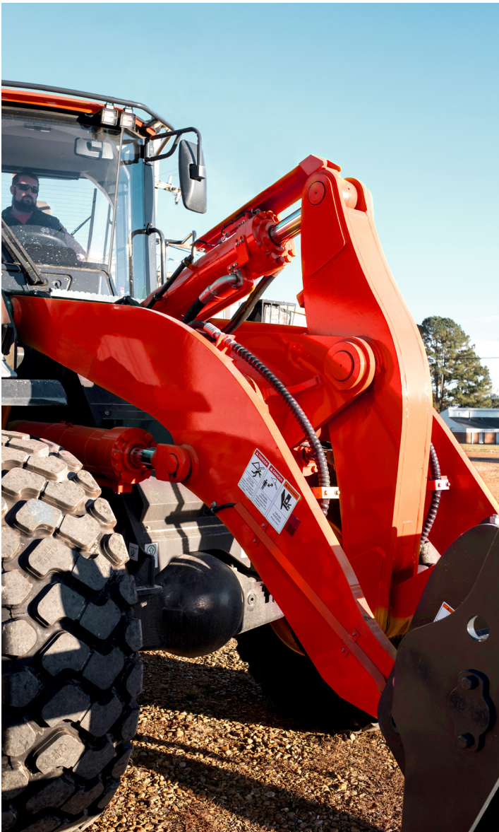
The Taylor T-1023 features optimized Z-Bar geometry that positions the bucket closer to the tires, achieving high bucket breakout forces with maximum rollback. The option of hydraulic quick coupler attachment adds versatility to Z-Bar machines, allowing use of multiple tools to suit the job-site needs.
