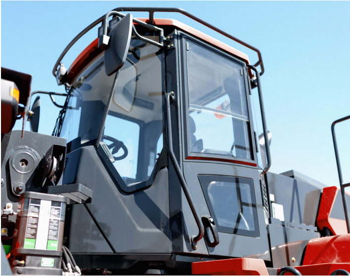
The Taylor T-1045 has been designed to offer optimized visibility. A panoramic view cab with curved front glass has been paired with well-positioned lift arms to allow the operator a clear line of sight to the attachment at ground level.
