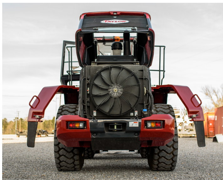
The rear full fenders swing out for easy access to the engine compartment. The electrically actuated, wide opening fiberglass hood of the Taylor T-1025 gives you easy access to the engine and its easy-to-reach service points. The radiator also swings out for ease of service.
