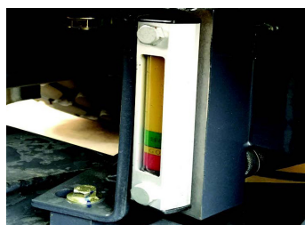
Autolube is a standard feature on the Taylor T-1025. All pressure taps and site gauges are easily accessible. Fluid drains provide environmentally friendly drainage capability and are grouped together for convenient serviceability.
