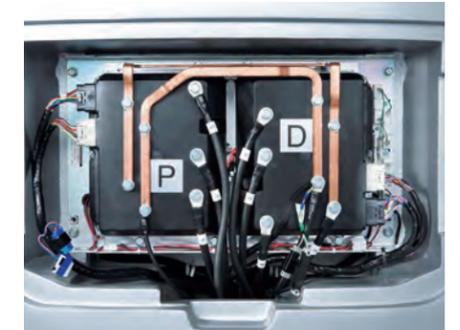
Remove rear panel for access to the controller for inspection and planned maintenance.
