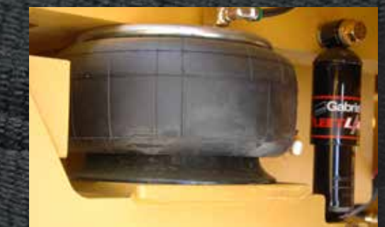
Firestone® air springs, stabilizing shock absorbers, and isolation mounts
