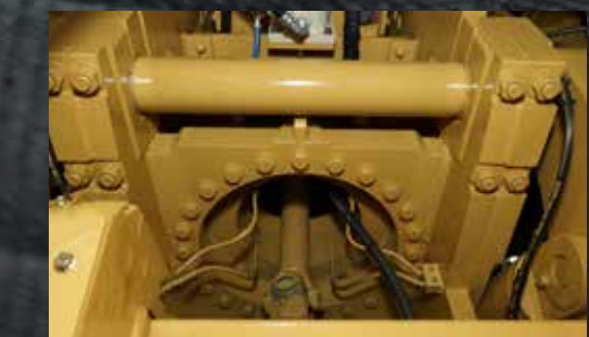
Heavy duty split mainframe with oscillating bearing frees axle pivot
