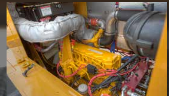
QSB-6.7 Liter Cummins Electronic Turbocharged Diesel Engine-Tier IV
